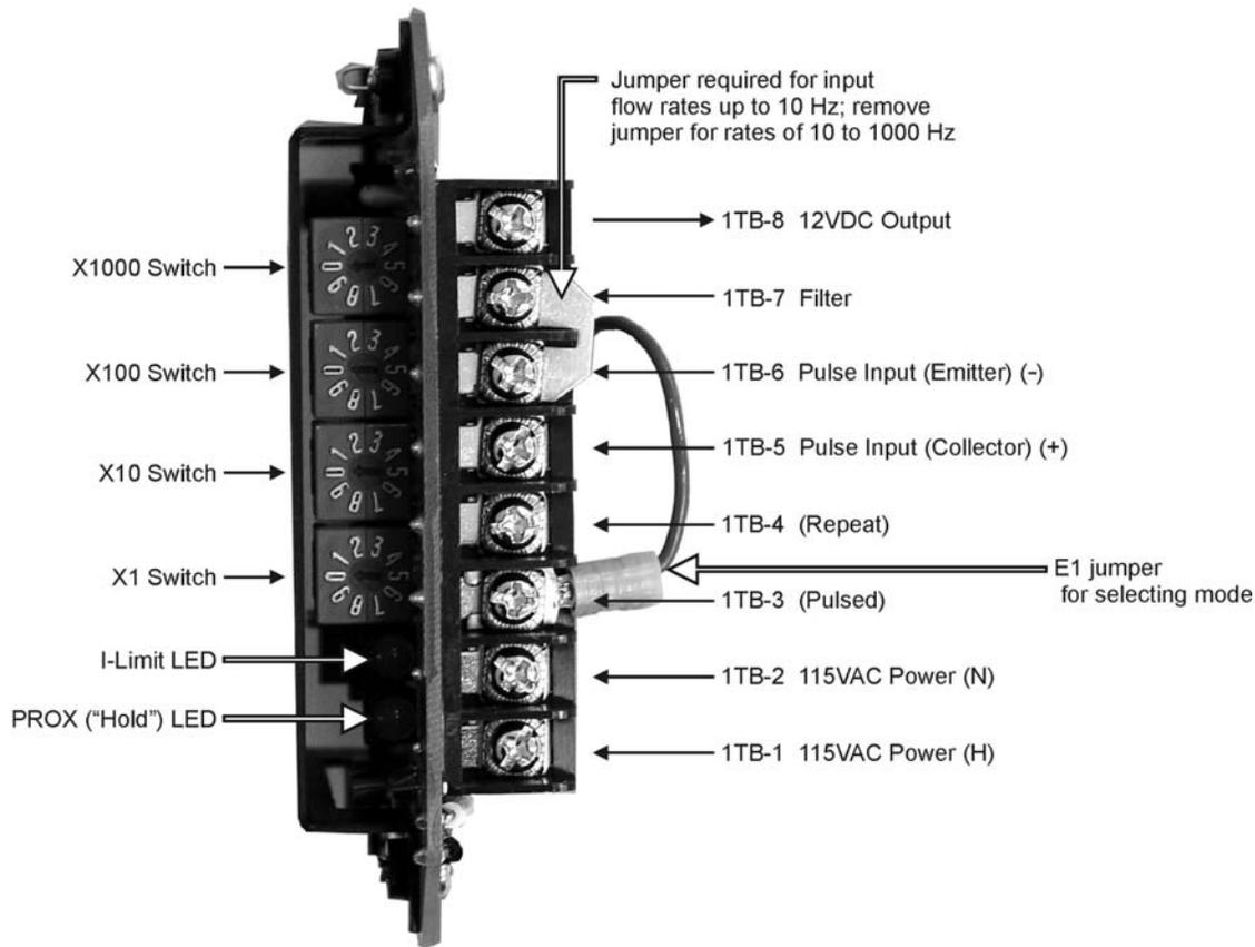
Figure 1—Field wiring of CD20A (115VAC) assembly
