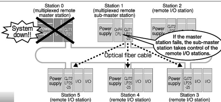
Note: The 'multiplexed' remote I/O system is a remote I/O system incorporating the 'redundant control' function.
