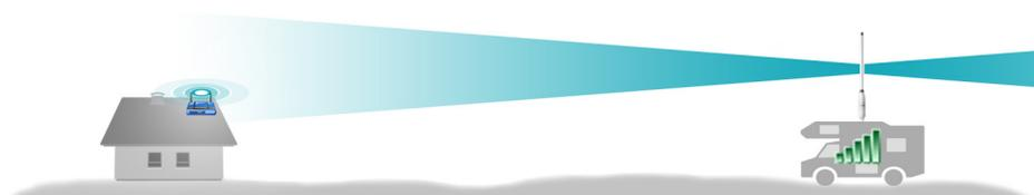
A wrong installation of the antenna will substantially reduce the maximum possible communication range.
