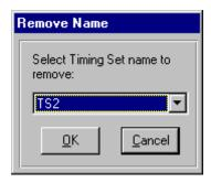
Names are added to the Timing Set and Table lists by importing them from external files or by entering them in the Parameter Pane. This dialog allows names to be removed that are invalid, misspelled or that no longer apply. These lists are used during validation to ensure that each subsequence references a known timing set and table.
