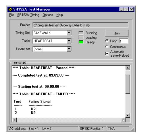
To use the Test Manager simply load a project file, select an appropriate timing set/table pair and press the Run button. Test results are reported in the Transcript window and operating status is indicated by LED-like controls.
