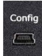
Insert mini USB cable onto Etrolink config port and connect other end to PC. When video server is powered on, Etrolink will not be operational. Once you are done working with Etrolink™ config port, remember to unplug USB cable from Etrolink™ config port.
