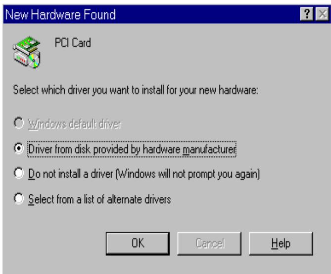
Choose the default option “*Driver from disk provided by hardware manufacturer*” and then a dialog box is shown to prompt you give the path of installation disk.
