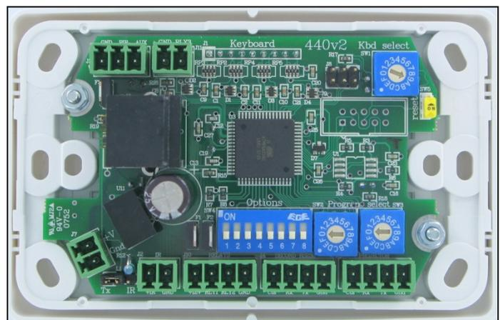
At the top left is three-terminal connection J3, with two inputs, one for the PIR input the other is unallocated at the moment. Next to it is connection J11 for Relay 3, a “power on”, USB switcher or aux screen/dipper relay drive.
