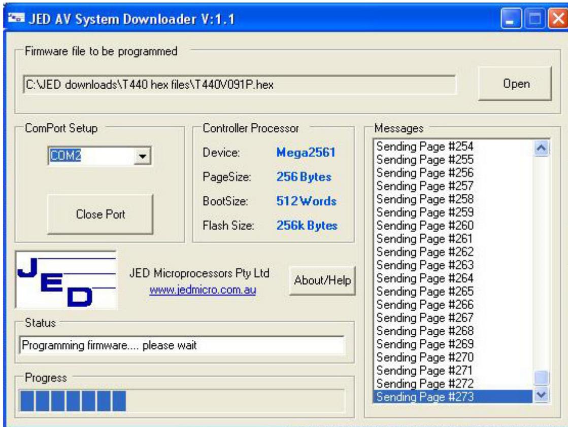
3. In the first window, “Firmware file to be programmed”, click on “Open”, move to the directory: “C:\JED downloads\T440 hex files”, and double-click on the latest T440Vxxx.hex file there. The “Messages” window should show “Open Firmware Hex File” and “Firmware hex File OK (and size) in bytes”;
