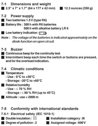
Note: This multimeter, of overvoltage category III satisfies the severe requirements of reliability and availability corresponding to industrial and domestic permanent installations (IEC 664-1). 7-5-2 Electromagnetic compatibility : conforms to CE Emission (EN 50081-1) Immunity (EN 50082-1)
