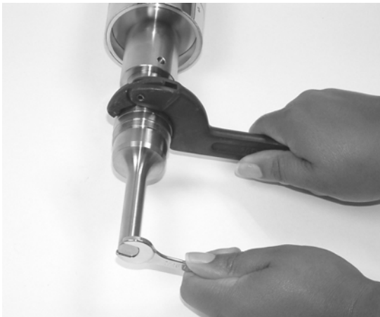
Figure 4.2 Connection or Removing Tip and Horn
