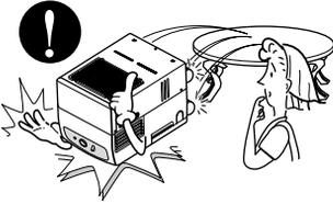
Be sure to replace bucket properly after emptying to prevent water from collecting on the floor.
