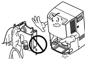
**Do not clean the dehumidifier while it is plugged in, especially if it is wet.**
