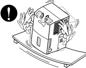
Do not install dehumidifier in an area where temperatures will fall below 65°F (18°C.)
