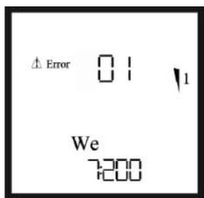
ERROR 01 means that no calibration procedure has been carried out. 7.200 seconds (2 hours) is the time remaining until the unit switches off, if it is not calibrated.
