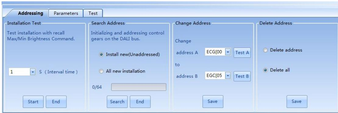
Select Short Address A of control gear that needs to be modified in Change Address bar **address A** **ECG[00]**, and modify to another specified Short Address B that has not been occupied **address B** **ECG[05]**. Then click **Save** to confirm current modification.
