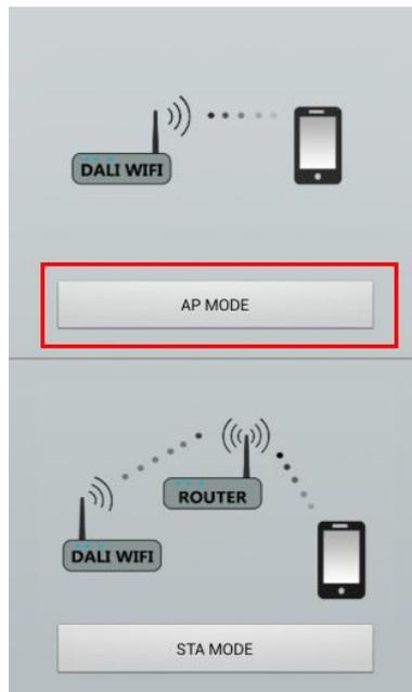
2) Return to Netmode (AP) setting interface and input a WIFI network name (SSID) eg. "DALIKWIFI" and input the Password and then click "Set" button. The whole setting needs 8s
