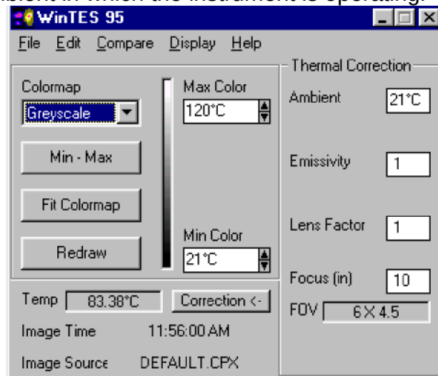
Fig. 7 WinTES Control Window with Thermal Correction Open
