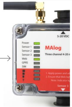
6. Check that the Sensor light blinks on power up. This will happen once and then read according to the sampling interval
