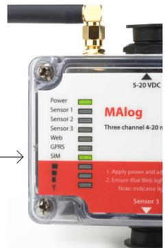
4. The GPRS light should then become active to indicate a successful connection to the GPRS network.
