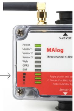
3. **The SIM light should then become active to indicate that a SIM card is detected. This should happen within approximately 10 seconds of start up, but please note that if the product has been shipped internationally, the SIM light may take several minutes to lock onto the local GSM provider network.**
