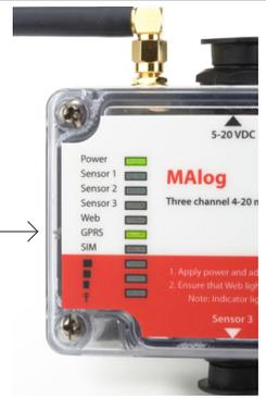
5. The Web light should become active to indicate a successful end-to-end connection with [MAlog.itmsoil.com](http://MAlog.itmsoil.com)
