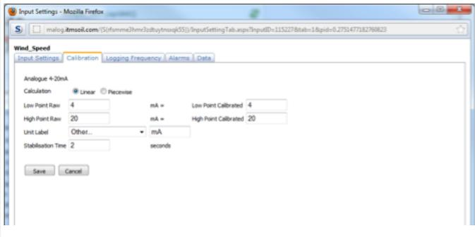
The Analogue calibration will allow you to set the raw high and low range, the calibrated high and low range, the desired unit label, and the stabilisation time which is the time in seconds the logger will wait after powering the sensor and before taking a reading.
