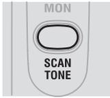
Press this button briefly to activate or de-activate the scan mode. Press and hold this button to activate or de-activate the current privacy code (CTCSS/DCS).
