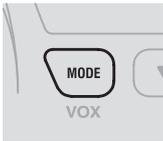
Press this button briefly to activate the function mode. Press the button again (repeatedly) to step through the function menu. Press and hold this button to activate or de-activate the VOX function.
