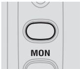
Press this button briefly to activate and de-activate the squelch level mode. Press and hold this button to activate or de-activate the MONITOR function.
