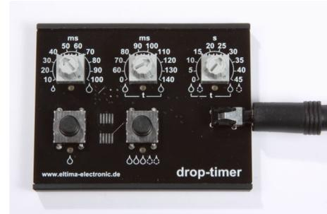
Due to the precision of the whole system, made up of the **drop timer**, drop dispenser and light barrier, the general form of the generated crests, pillars, umbrellas etc. will be fairly much the same for each release.
