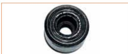
interior ring damaged for 100%
