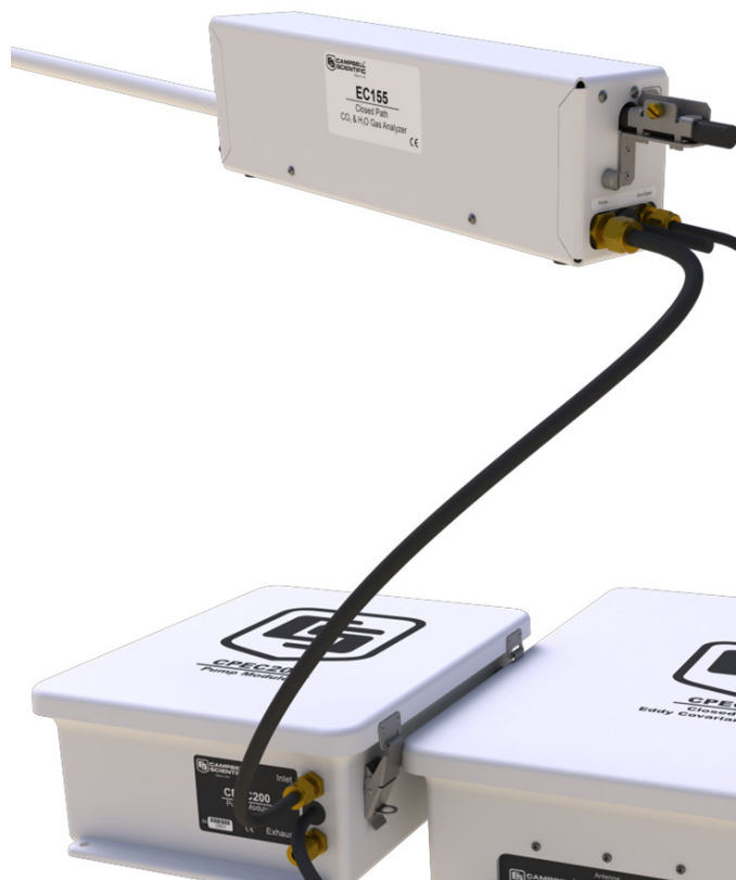
FIGURE 5-5. Connecting pump tube from EC155 analyzer to pump module
