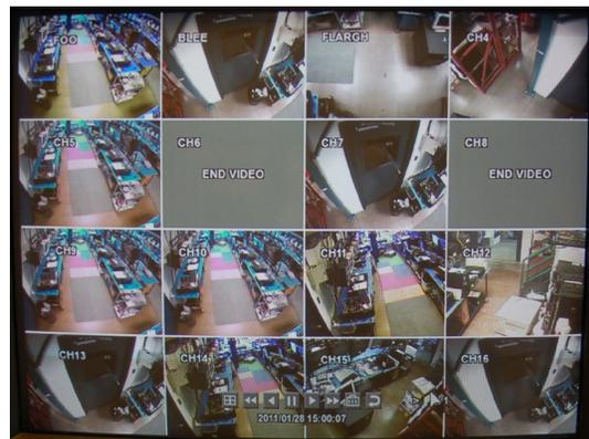
Turning steadily counter-clockwise will reverse play by up to 64 times. When the SHUTTLE WHEEL is released, playback is paused.
