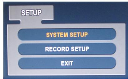
To setup the recording behavior of the DVR, highlight RECORD MENU and press ENTER.
