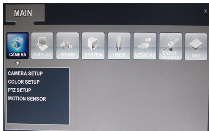
To navigate the setup menu, use the CURSOR KEYS and the ENTER and RETURN buttons. In general, the ENTER button is used to select and change a particular item and the RETURN button is used to cancel a change or exit from a particular setup screen.
