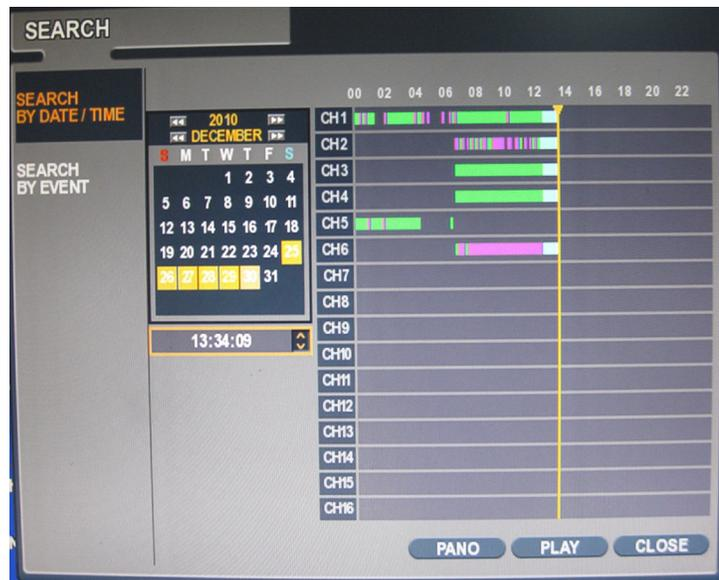
The DVR uses a calendar and timeline search method for quick access to recorded footage. The calendar displayed on the left shows the current month. Days highlighted in yellow have recorded footage. The timeline on the right shows a 24 hour status of all channels for the selected day.
