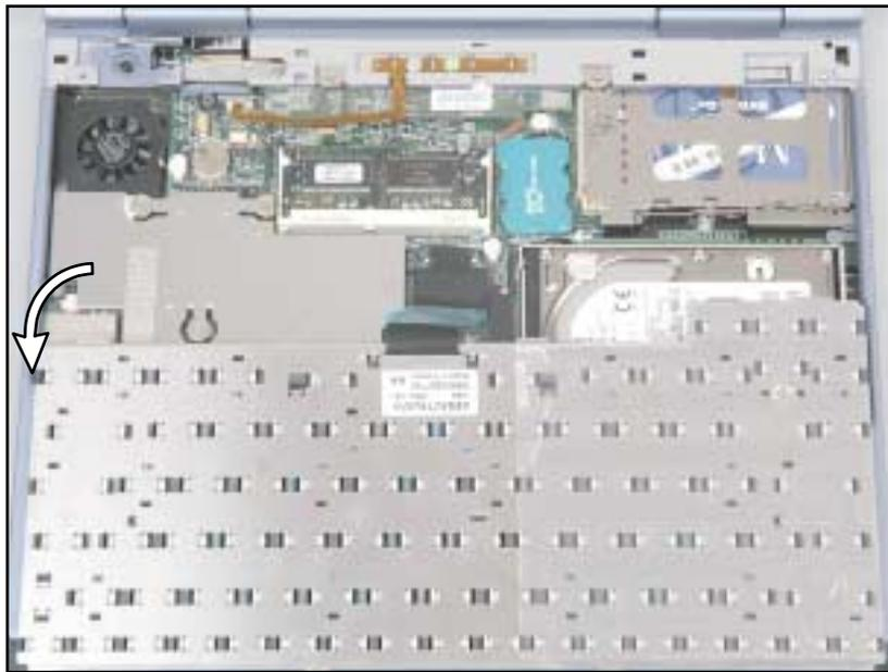
Removing the keyboard exposes the following replaceable components:
