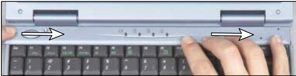
The bezel is correctly mounted when each end is flush with the notebook case and the bezel is flat all the way across. If the bezel is not flat, you should follow “Removing the keyboard” on page 137 to remove the bezel again, then follow Steps 7-8 to replace the bezel.
