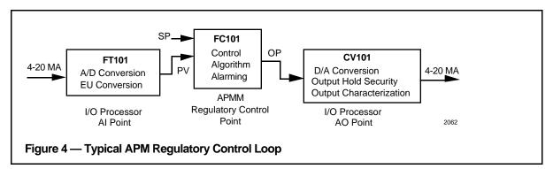
and alarming. This partitioning of functions allows more efficient use of APM capability and provides for I/O expansion.
