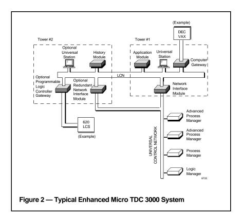
Also supplied as standard nodes with all Enhanced Micro TDC 3000 systems are an AM (Application Module) and a US (Universal Station)<sup>2</sup>, both of which are also housed in Tower #1, and an HM (History Module) which is installed in Tower #2.
