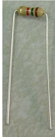
Figure 9: 1.5 K \Omega resistor with leads bent down.
