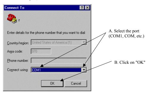
6. Set the COM port parameters. The following assumes that COM1 port is used and HyperTerminal is set to the 34970A's default configuration.
