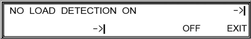
**Fig. 35: Display of the OPTION no load detection: ON**
