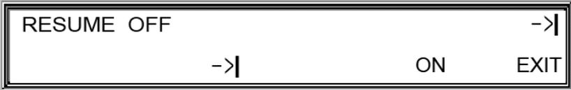
**Fig. 38: Display of the OPTION resume run: OFF**
