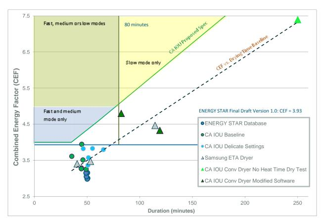
Figure 2: Tier 1 California Investor-Owned Utility (CA IOU) proposed specification for conventional residential clothes dryers (CA IOU 2013b).
