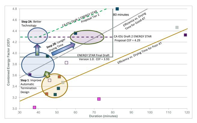
Figure 3. Potential design improvement options required to achieve efficiency gains (AT is automatic termination) (modified from CA IOU 2014).
