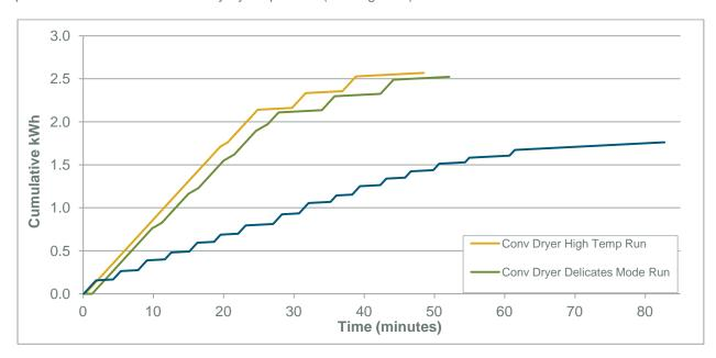
Figure 1: Cumulative energy consumption over time for full size conventional dryer across different drying modes (CA IOU 2013b).
