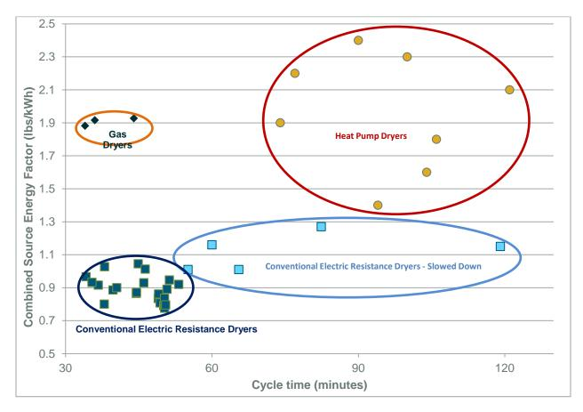
Figure 5: Source energy of gas, heat pump, and conventional dryers (original research).
