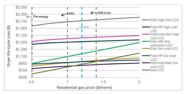
Figure 6. LCC of different dryer technologies with different energy prices (original research).
