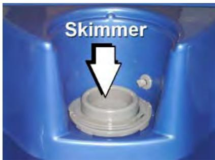
To clean the skimmer filter, remove the access lid that covers the entire filter area. Lift the center float of the skimmer assembly until it is fully extended. Hold the centerpiece of the assembly and turn it counterclockwise until the flats of the basket are aligned with the securing tabs. Then pull the basket assembly straight up to remove it.
