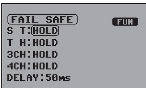
In this menu, you can make the Fail Safe settings individually for each channel. This function sets the servo of the respective channel into a predefined position, in case of a signal loss of the receiver. For instance, the throttle servo of an engine-powered model can, in this case, be set to idle (of an electric-powered model to motor Off), so the model does not move on without control.
