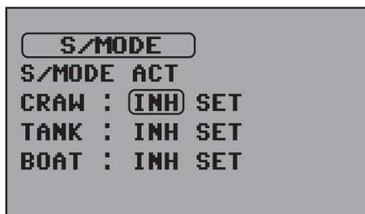
In this menu, you can select preprogrammed mixers for the various model types (crawler, track vehicle, boat), which are tuned for the characteristics of the vehicles. After activating the function, further settings can be made in the menus: After you switched from **INH** to **ACT** in line **CRAW**, **TANK** or **BOAT** in column **ACT**, you change to **SET** and confirm with **ENTER**.
