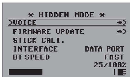
You can enter HIDDEN MODE from the main screen, by pressing the **UP** and **DOWN** buttons simultaneously. Here, you can load the voice files or a firmware update from the SC card. You can also do the stick calibration.
