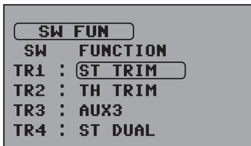
In this menu, you can assign a function to trim buttons, switches and rotary controls. By default, some buttons and switches have already been assigned functions, which can be assigned again as all the others, as follows: After selecting a switch with the **UP/DOWN** buttons, press **Enter**, and the menu with the possible functions for this switch appears.
