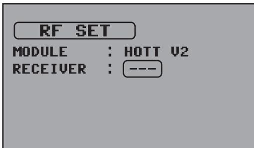
This menu appears if no receiver is bound to the selected model memory location. After the binding process, the whole menu appears as on the following display.
