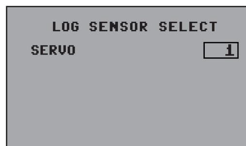
Here, the devices are displayed whose data are output via the Bluetooth interface, in order to display them e.g. in the Live Log of the Firmware Upgrade Studio. To do so, the optional Bluetooth module S8351 has to be used. The settings for the data transmission are made in the Hidden mode (see Chapter Hidden mode).
