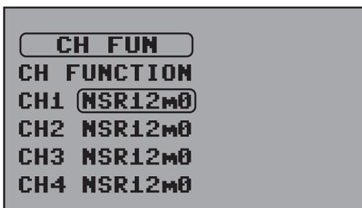
In this menu, the properties for adjusting to the servo, used by the respective channel, are set. **(Observe the information from the servo manufacturer)**
