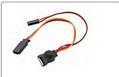
Connect the adapter lead 7168.S to the USB interface order no. 7168.6. The connectors are reverse polarity protected: note the small chamfers on the sides. Never use force – the connectors should engage easily.
