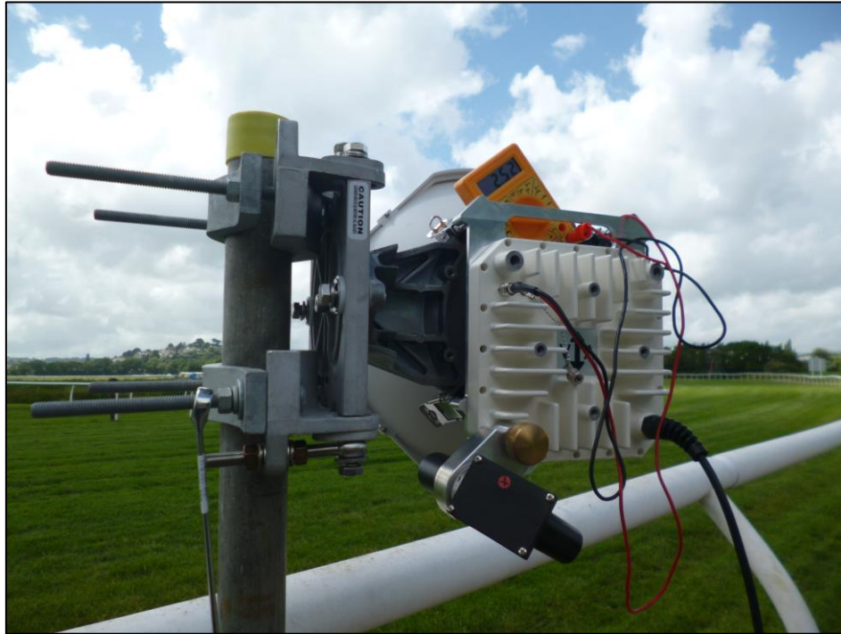
Figure 24 - E1000e with 30cm dish using alignment scope from V100 / V1000 radios
