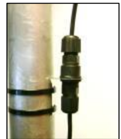
Figure 21 - RJ45 Seal Kit installation
