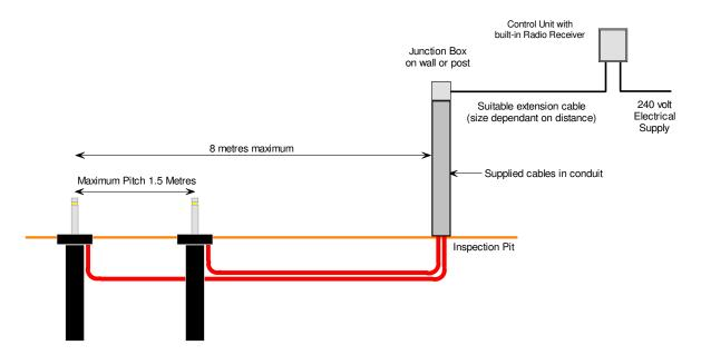
A separate duct must be run from each GENIE MKII bollard to the edge of the carriageway. The furthest bollard must be within 8 metres of this position.
