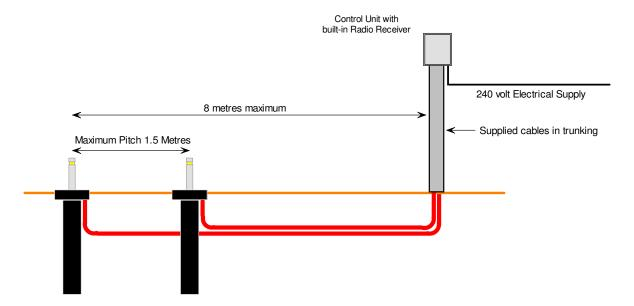
A separate duct must be run from each GENIE MKII bollard to the control unit location. The furthest bollard must be within 8 metres of the control unit.
