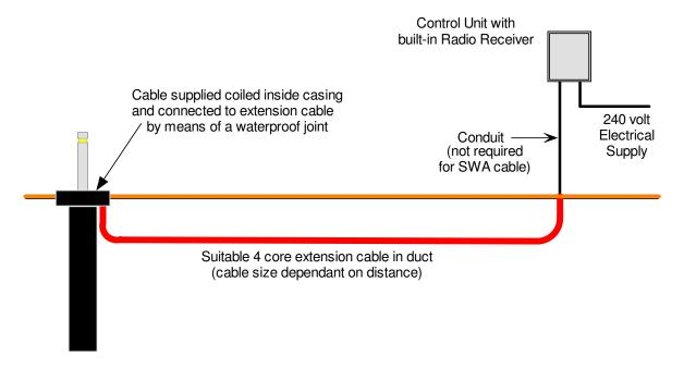
The length of 4 core cable supplied with the GENIE MKII unit must be carefully coiled up within the bollard housing. There is ample space within the housing to do this.
