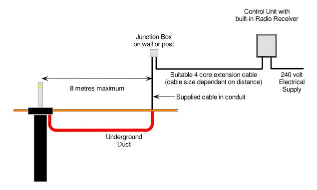
The length of cable supplied with the GENIE MKII unit is run to a junction box within 8 metres from the bollard. The necessary length of extension cable can then be joined within the junction box. The extension cable can then be taken to the control unit position. All wiring must be in accordance with current electrical regulations.
