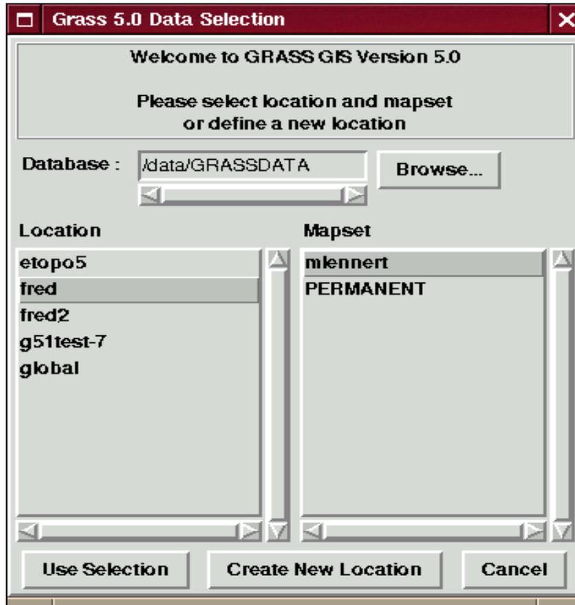
Click on the button "Create New Location" which will get to the above text screen on which you can enter a non-existing location name and continue with **ESC-RETURN**.
