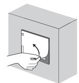
2) Peel the release paper off the back of the new protective sheet. Position the hole for the USB environmental protection cover of the protective sheet to the USB environmental protection cover of the GOT. If the protective sheet without the hole for the USB environmental protection cover is attached, position the sheet from the upper left of the GOT.
