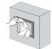
To attach the protective sheet, attach it from one direction gradually. Make sure to fit the protective sheet onto the joining surface closely without leaving any air between the protective sheet with adding additional pressure sufficiently to the Attach the protective sheet with adding additional pressure sufficiently to the adhesive side of the outer circumference. To hold adequate strength of the adhesive joining, use the GOT after a lapse of about 24 hours.
