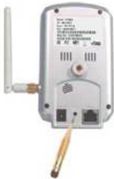
Figure 3-22: Stick on the reset button to set to the factory default
