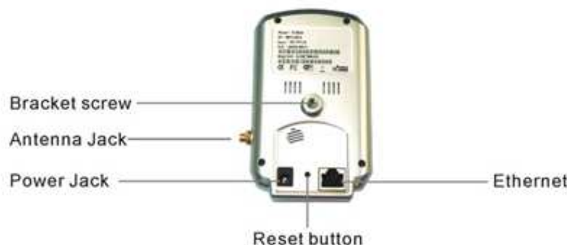
Figure 2-2: Major components in the back panel
