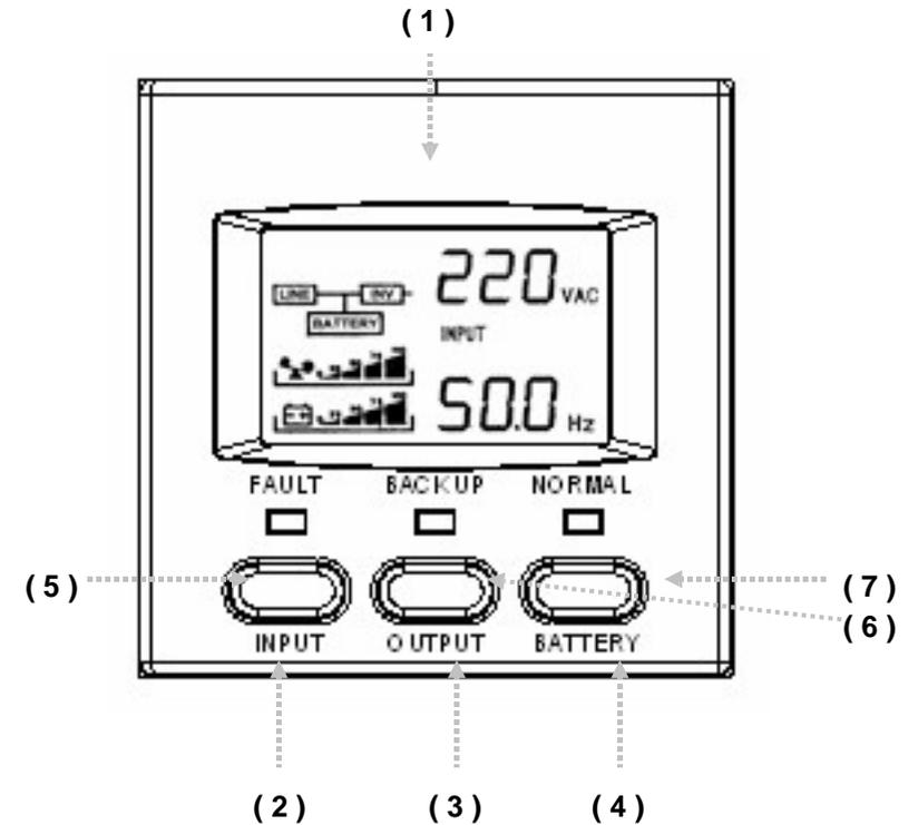
1. LCD Display: indicates the UPS operation information, including UPS status, input/output voltage, input/output frequency, battery capacity, output load, temperature, etc.
