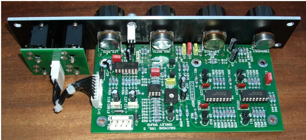
*This is the issue 5 Oakley Equinoxe behind a black finish Schaeffer panel. Note the use of the optional Sock4 socket board to facilitate the wiring up of all those sockets.*
