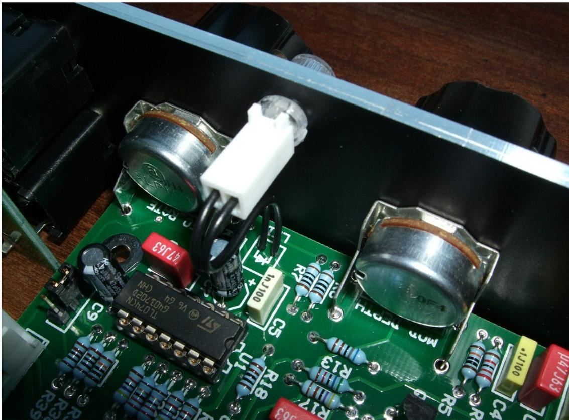
*Using a two way Molex KK housing to connect the bi-colour LED to the circuit board. The LED is held onto the panel with a clear Cliplite lens, or equivalent.*
