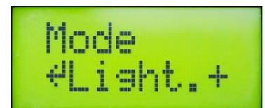
The status "Backlight" is stored in non-volatile memory, and will be automatically applied when you turn on the power.
