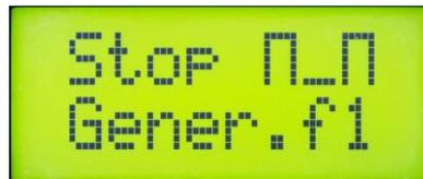
In this example showed state of stopped generation. After starting will be generated square signal with f1 frequency
