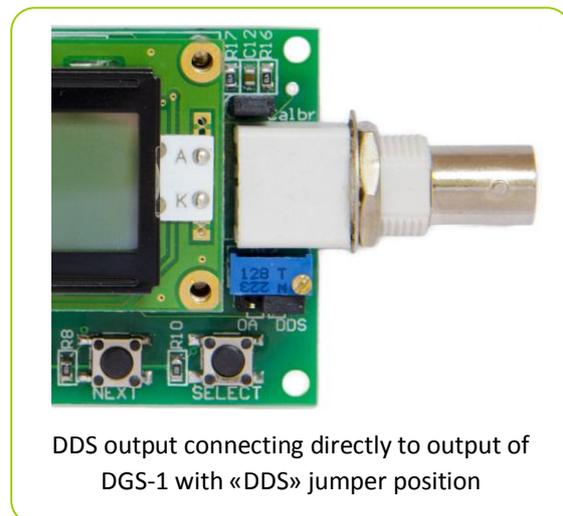
At the "OA" position signal arrives to the output connector through the operational amplifier. Gain of operational amplifier is adjustable by the potentiometer. In this case, the peak voltage of generated sinusoidal or triangular signal from the amplifier output can be up to 4.6 V. Voltage peak-to-peak square wave is 0,1 to 4,6V, and does not depend on the gain of the operational amplifier.
