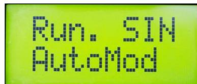
In this example, DGS-1 is in generation state. It is do generate sinusoidal signal with FSK modulation
