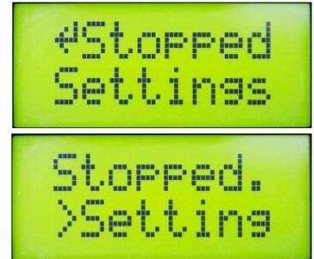
If the DGS-1 is in generation state (the "Stopped / RUN" menu parameter is "RUN"), then when you change a menu setting, the signal changes instantaneously, in accordance with the specified parameters. If the device is in the "Stopped" state, the changed parameter will be applied when next starting.
