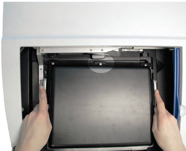
Fig 3-7. Inserting the cassette
