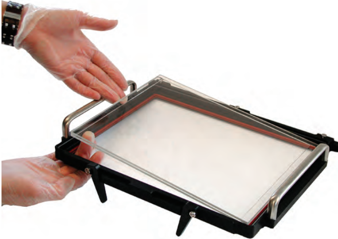
Fig 3-3. Inserting plates in a DALT Cassette.
