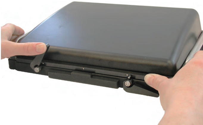
Fig 3-4. Closing the cassette locking cams.
