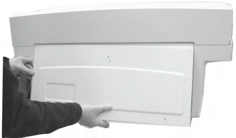
Fig 7-3. Removing the rear pane
