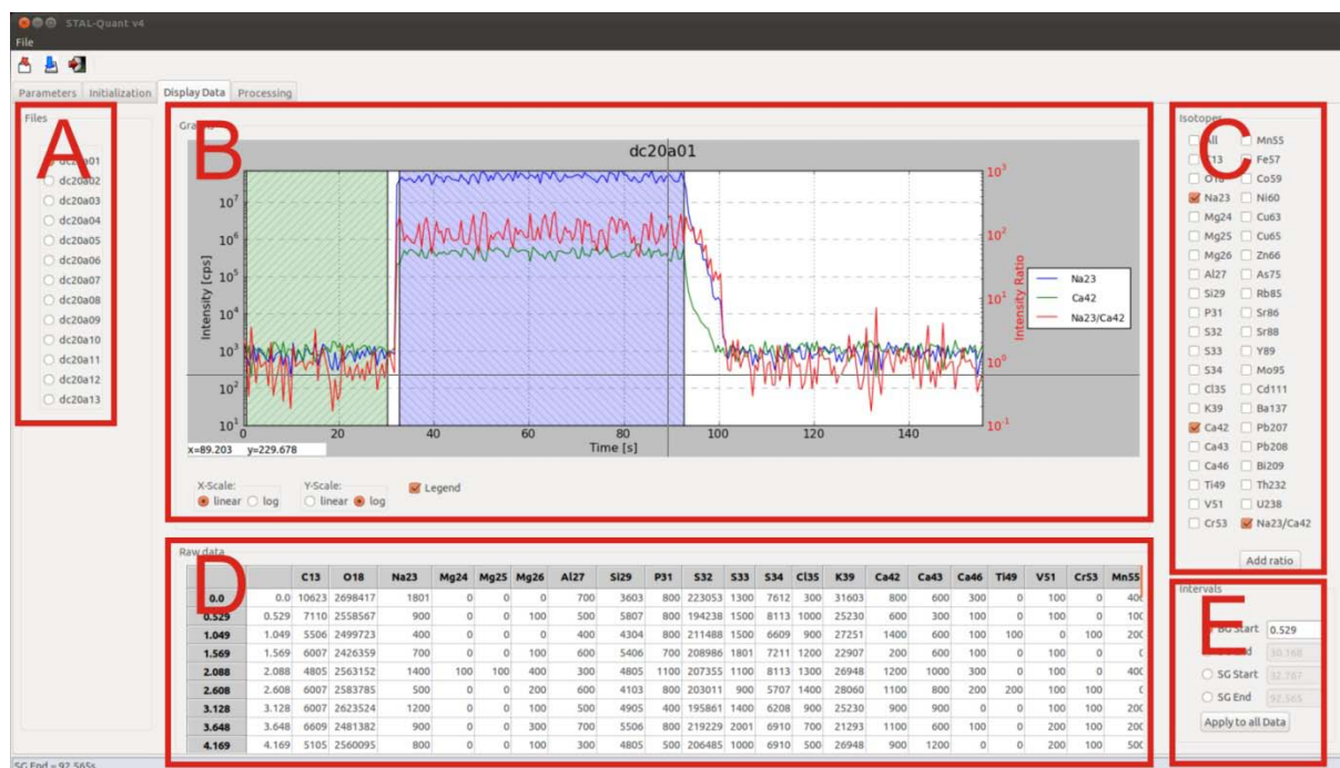
Figure 23: The display tab comprises a list of the imported data files (A), the plot area of the selected data file (B), the list of the isotopes to be plotted (C) including a function to generate and plot isotope ratios from the raw data, a table of the raw data (D) of the selected data file, and the selection of the interval variable to be changed (E). Ablation intervals can be chosen by clicking either in B or D, as well as entering time values manually in E.
