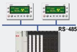
Thanks to multi-master function, XGT Panels can control and supervise one single system.
