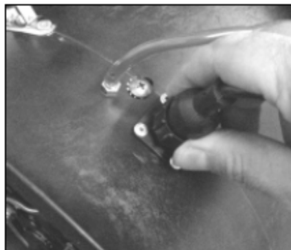
Figure B-13: Connect Controller to Duct Blaster Fan
