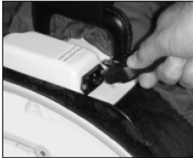
Figure B-7: Connecting Power to the Blower Door Fan
