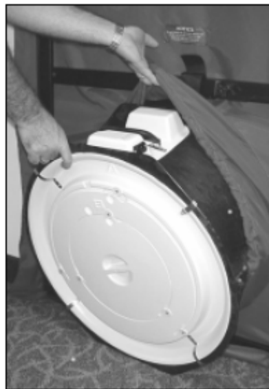
Figure B-3: Installation of Blower Door Fan
