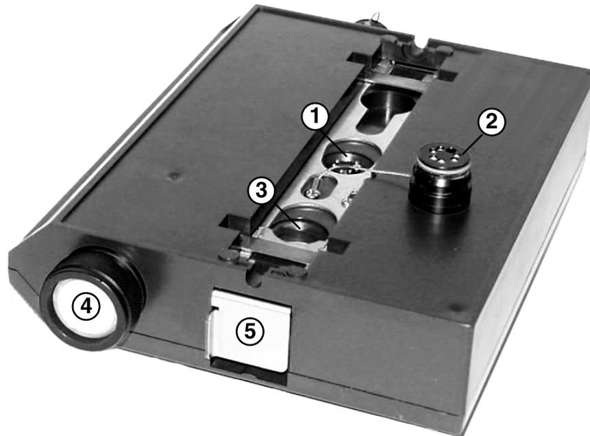
Figure 1-3 Field Wizard Components - Bottom View
