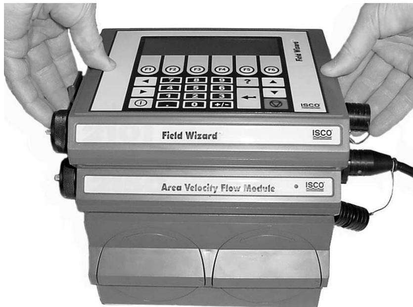
Figure 3-3 Field Wizard Connected to a 2150 Site
