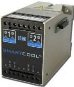
Each channel is provided with an external 12VDC (-) output for the control of an external relay during save cycles. The relay for each channel is utilized for the slide valve control function. In Analog Output mode, the relay of channel one can be used to drive an external relay for switching the IIM signal in place of an existing signal (i.e. BMS) when required.
