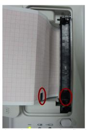
Reload the paper in the paper tray, close the paper casing firmly. If the problem still exists, please contact the manufacturer or the local distributor for further disposal.
