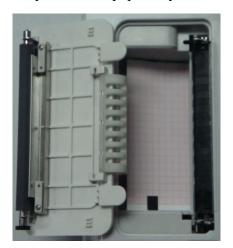
**Note:** If the paper with paper markers is used, make sure that the markers are on the bottom.
