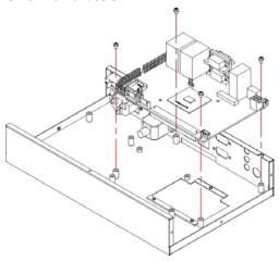
2. Use four screws install SBC with front panel.
