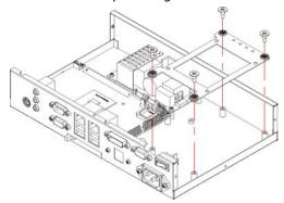
2. Install the holding bracket with HDD, then re-install HDD drive bay back to chassis.
