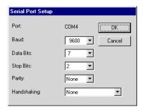
**5** Enter the *Baud* rate, *Data Bits*, *Stop Bits* and *Parity* and *Handshaking* settings for the device.
