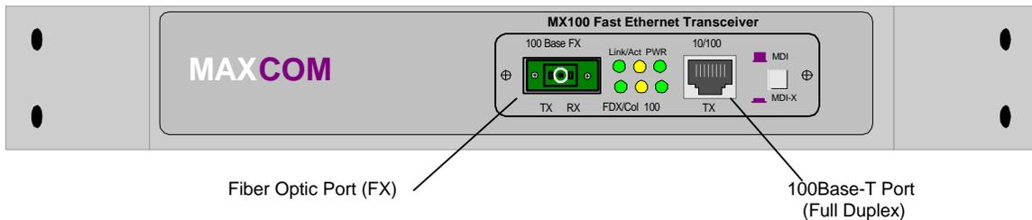
**Figure 2: Front Panel of MX100**
