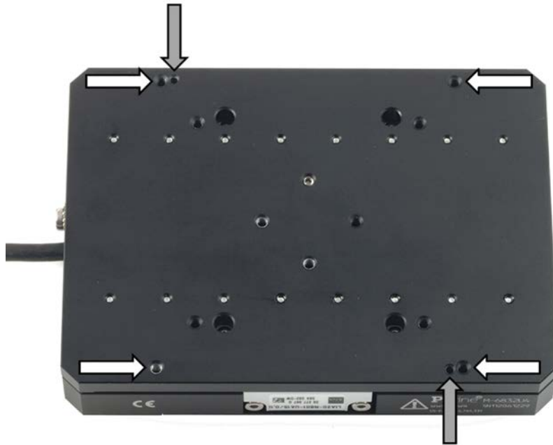
Figure 8: Holes to be used for screws (white arrows) and locating pins (gray arrows) in the lower M-683
