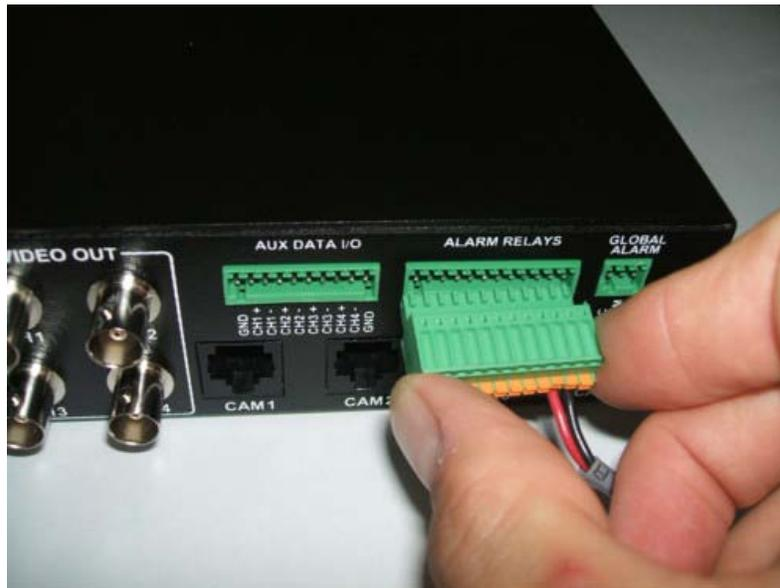
**Figure 11: Connect alarm inputs into the DOG VPDA alarm relay outputs**
