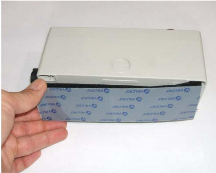
**Figure 3: Mounting with velcro**
