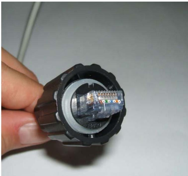
**Figure 6: Slide backshell over RJ-45 connector as far as possible**
