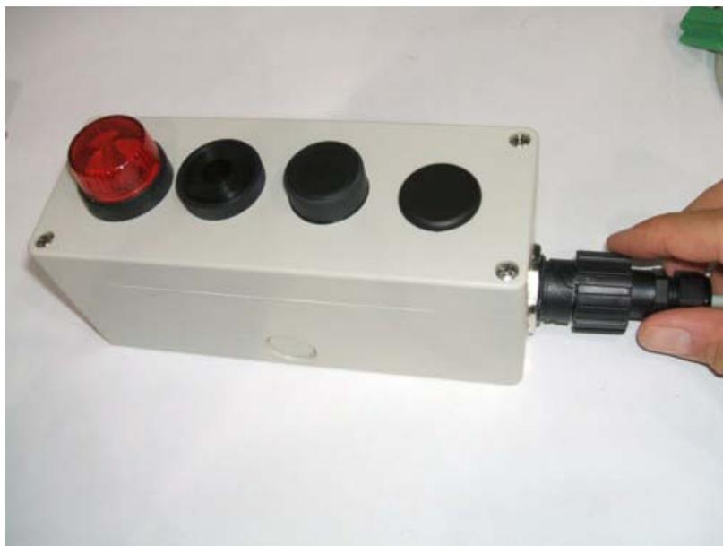
**Figure 10: RJ-45 connection for the duress alarm module**
