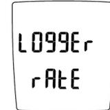
The display will advise you to input a new sampling rate. To change the sampling rate, press  or  until the desired rate is displayed. Press  to confirm the value.
