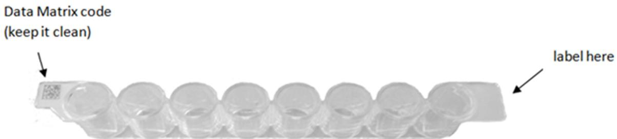
Avoid contact of data matrix code with organic solvents! The ArrayMate needs the information encoded in the data matrix to perform the assay and the analysis afterwards.
