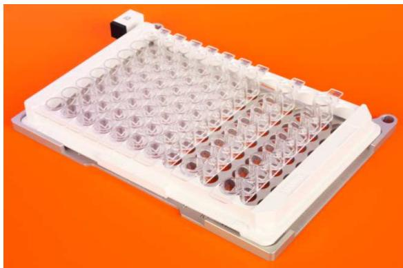
ArrayStrip frame with strips inserted in accordance with the Worklist.
