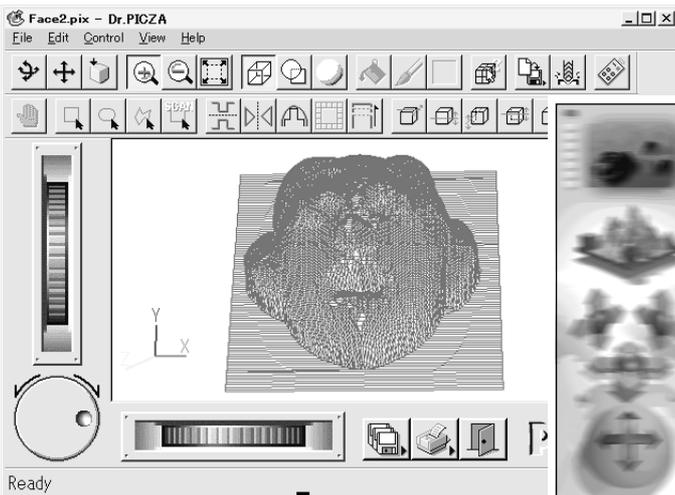
**4** Launch the 3D graphics application and import the DXF file. Make the pyramid and arrange the face and the pyramid using the layout shown below.
